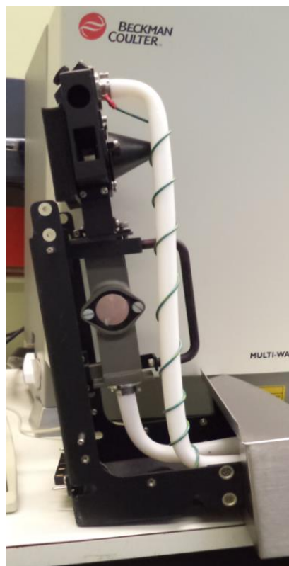
Figure 19: The sample cells, the water in- and outlet (white hoses). This part of the instrument was taken out of the machine to take a photo
